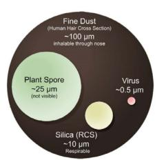
Silica dust ranges in size and is characterized by its jagged crystalline form.
